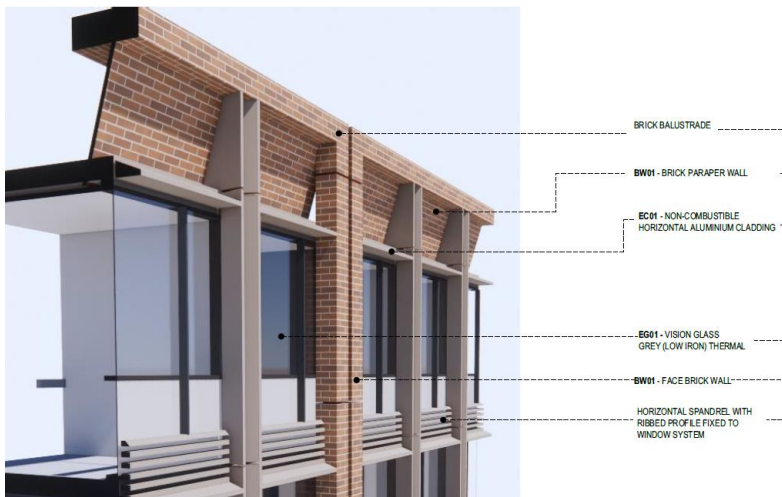
Figure 68: Proposed tower parapet detail showing canted wall
