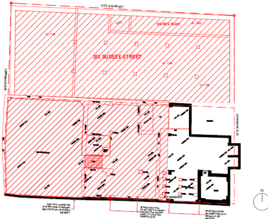
Figure 29: Proposed Demolition Plan Lower Ground
