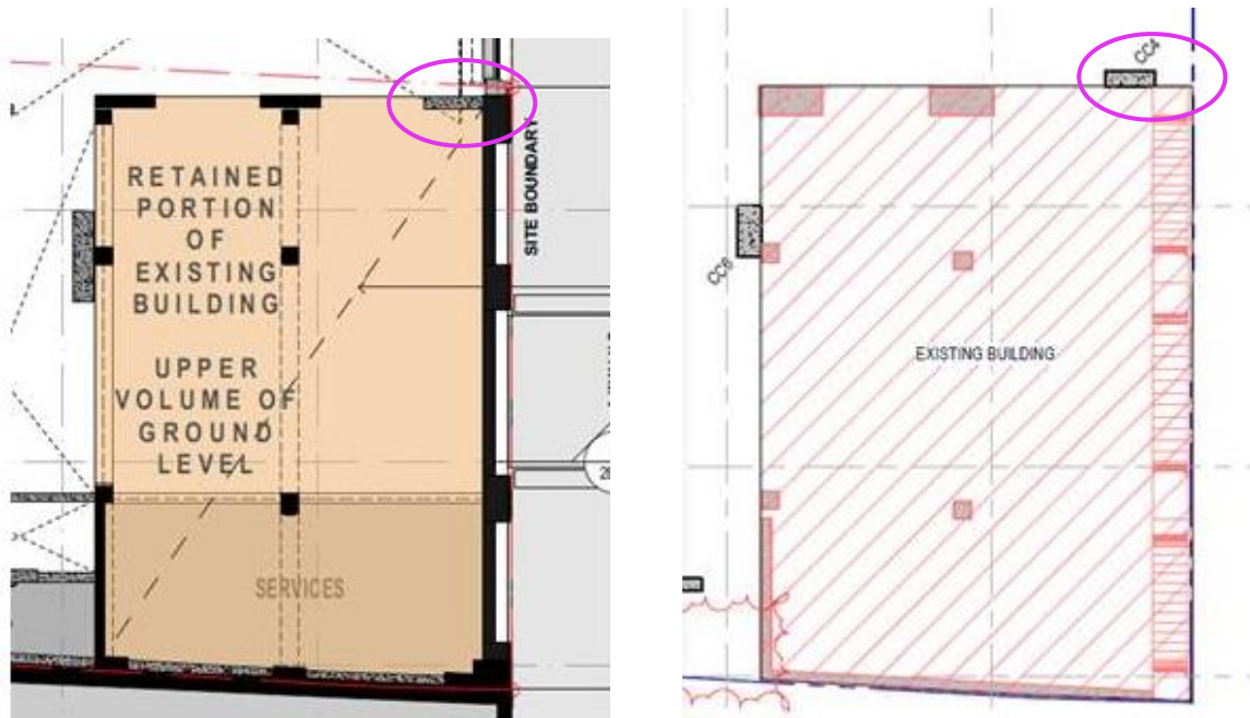
Figure 65: Proposed Level 1 Floor Plan (left) and extract of the Level 1 Floor Plan from the Structural Report prepared by Van Der Meer (right)
